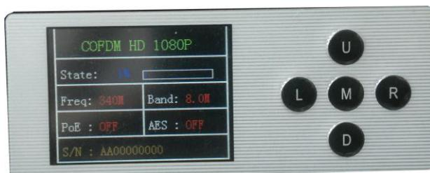
**Note:** when turn on the receiver, the LCD will blink to identify the wireless signal, receive the signals success, the **State** will be show green 100% scaling indicator. If can not receive the signals, the State will be show blue00% scaling indicator.
